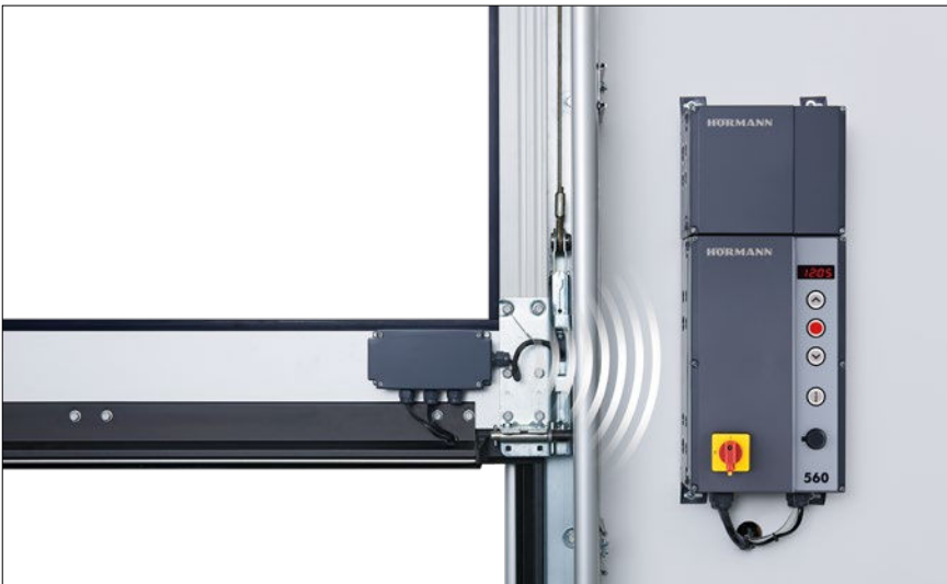
Radio transmission unit To transfer the signals from the door leaf to the control via Bluetooth (no coiled cable), power supply via a powerful battery; connectable components: optosensors LE (low energy), leading photocell VL1-LE/VL2-LE, 8k2 strip, rope failure device, wicket door contact, night latch contact
