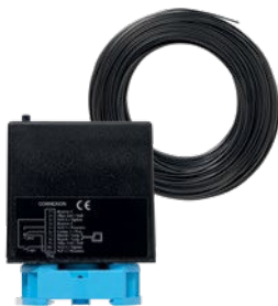
Induction loop Induction loop detector with normally open contact and change-over contact, can be set to pulse or permanent contact, direction recognition, 50 m loop cable
