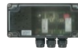
2-channel relay receiver HET-E2 24 BS 2 volt-free relay outputs for choosing the direction, one 2-pin input for volt-free OPEN / CLOSE limit switch reporting (for querying the door position)
