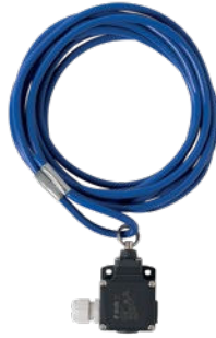
Pull switch with cord Horizontal or vertical fitting possible, aluminium die-cast housing IP 65, cord length 4 m
