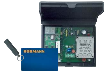
Transponder key switch TTR 1000-1 For 1 function via transponder key or transponder card; up to 1000 keys or cards can be saved Dimensions: 80 × 80 × 15 mm (W × H × D); decoder housing: 140 × 130 × 50 mm (W × H × D); switching capacity: 2.5 A / 30 V DC; 500 W / 250 V AC
