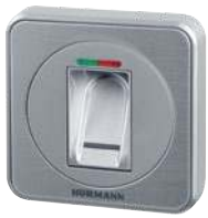
Finger-scan FL 150 For 2 functions, up to 150 fingerprints can be saved Dimensions: 80 × 80 × 13 mm (W × H × D); decoder housing: 70 × 275 × 50 mm (W × H × D); switching capacity: 2.0 A / 30 V DC
