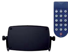
Radar movement detector RBM 2 For OPEN impulse with directional recognition, max. fitting height: 6 m; optional remote control for radar movement detector Dimensions: 155 × 132 × 58 mm (W × H × D); contact load: 24 AC / DC, 1 A (resistive load); protection category: IP 65
