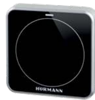
Transponder key switch TTR 1000-1 For 1 function via transponder key or transponder card; up to 1000 keys or cards can be saved Dimensions: 80 × 80 × 15 mm (W × H × D); decoder housing: 140 × 130 × 50 mm (W × H × D); switching capacity: 2.5 A / 30 V DC; 500 W / 250 V AC
