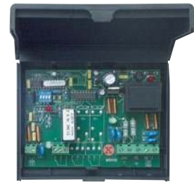
Decoder housing For code switches CTR 1b-1, CTR 3b-1, CTV 3-1, CTP 3 Dimensions: 140 × 130 × 50 mm (W × H × D), Switching capacity: 2.5 A / 30 V DC 500 W / 250 V AC
