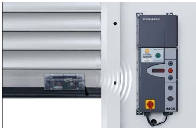
Optional: Radio transmission unit For transmission of signals from the door curtain to the control via Bluetooth – instead of a coiled cable. Power supply via a high-performance battery. For controls: 445 R / 460 R
