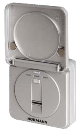
Radio finger-scan FFL 25 BS For 2 functions and up to 25 fingerprints, with hinged cover, recessed and surface-mounted fitting possible, plastic housing painted in RAL 9006 White aluminium
